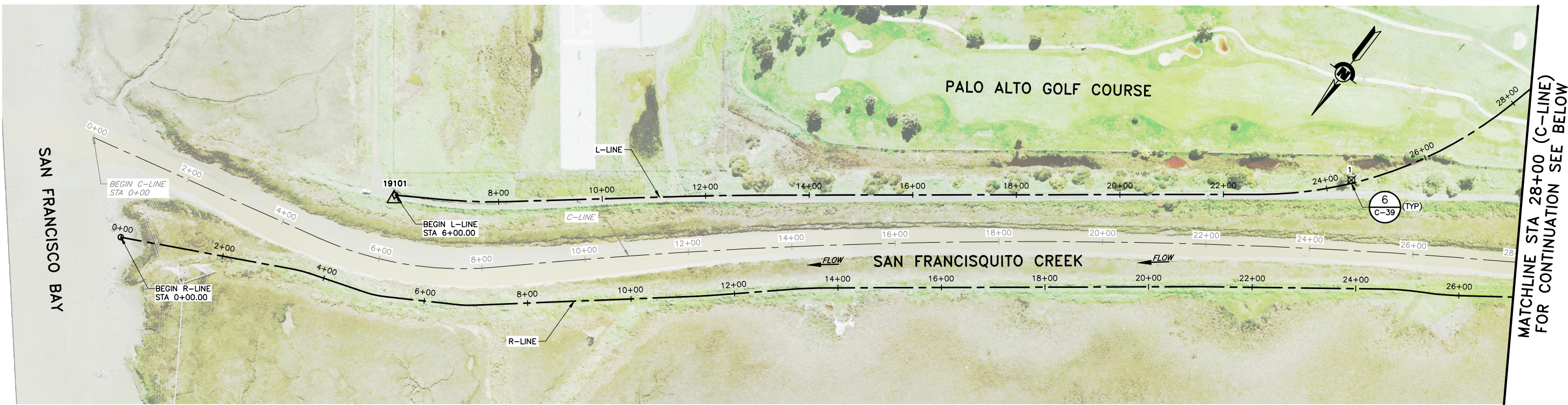
SURVEY CONTROL POINTS, SETTLEMENT PLATES PLAN SCALE: 1"=100'
